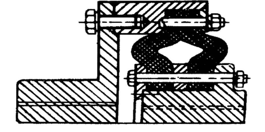
HI-TECH HDC Diaphragm Type flexible Couplings are long life & multi-directional couplings and have high tortional flexibility. Typical applications includes locomotive drives, compressors, pumps, Diesel Gensets etc.
